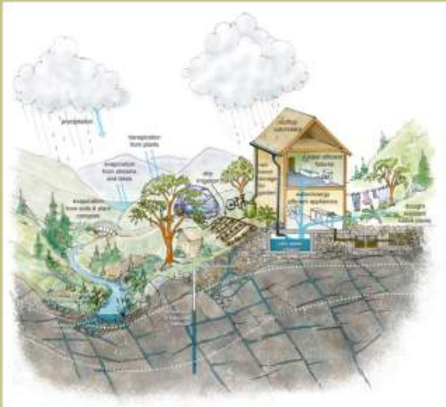
Schematic diagram (from 2008 Highlands Community Green Map) showing the hydrologic cycle of a rural watershed sitting on a fractured bedrock aquifer: precipitation, evaporation, transpiration, surface runoff and wetlands, and movement of groundwater through soil and cracks in the bedrock). Narrow strips (called "lineaments") containing more abundant and larger cracks lie beneath and along valley bottoms: Plus examples of proven household water conservation practices (efficient indoor fixtures and appliances, drip irrigation, rainwater and gray water harvest and storage, drought-resistant landscaping).
